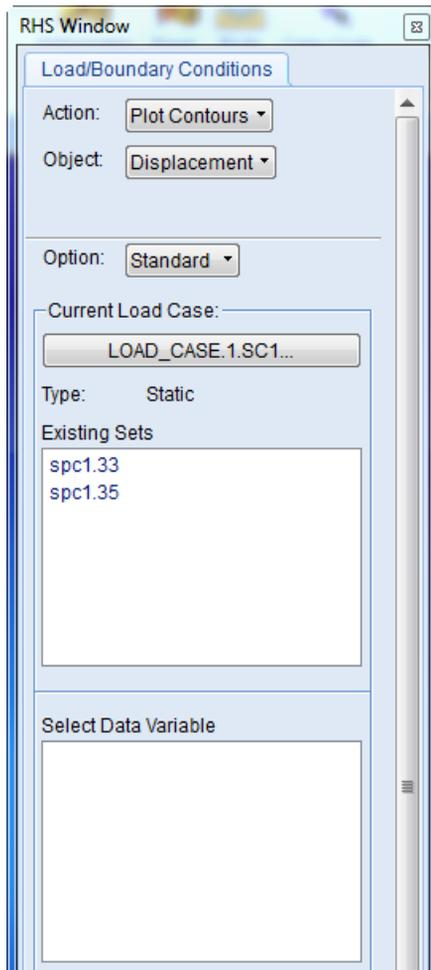
The spectrum values and color coding for these contour displays will span the range of values by default, but can be modified using the Display --> Spectrums menu. When you no longer wish to display this contour plot, select the Reset Graphics button on the Plot Contours menu form.
