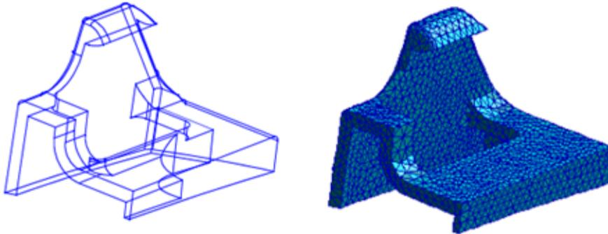
Figure 5-1 A geometry model versus a finite element representation
