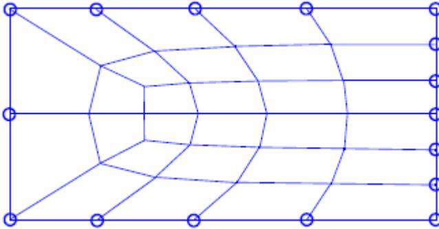
Figure 5-5 A mesh transition using mesh seeds
