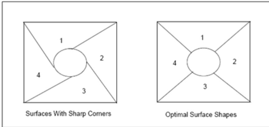
Figure 4-6 Surfaces with and without sharp corners
