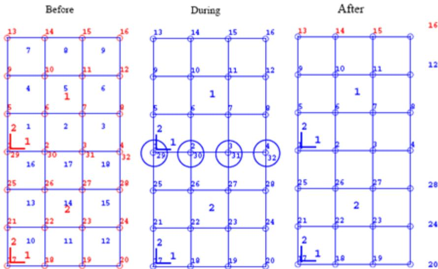
You have the option of equivalencing all nodes in a region, or just those nodes corresponding to a specified group or list, as discussed in Chapter 2 of this guide. Once the requested nodes are equivalenced, all references to the original higher numbered nodes (such as element definitions, loads, and boundary conditions) are automatically changed within Patran to reflect the new equivalenced node numbers.
