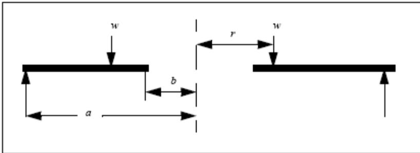
Figure 1-1 Representation of the Annular Plate
