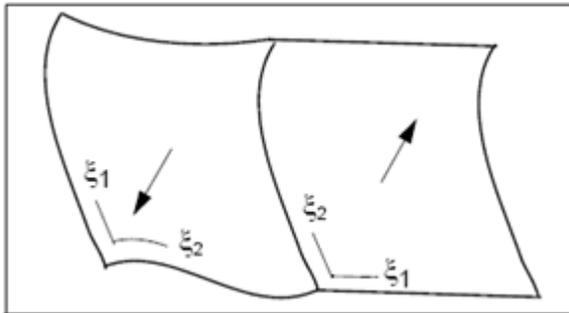
Use the Geometry application's Edit/Surface/Reverse form to display the surface normal vectors, and to reverse or align the normals for a group of surfaces. This form has a button labeled Draw Normal Vectors that displays the positive surface normal vectors within your display. Alternatively, the Show/Surface/Attributes form can be used to display these normals.
