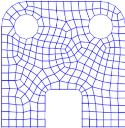
Figure 5-3 Example of Paver mesh technique
