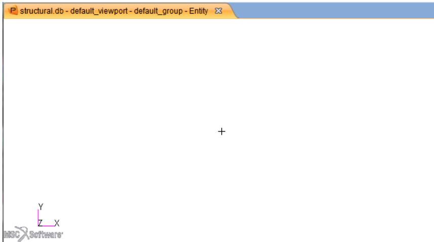
The top of the viewport lists the name of your database (in this case `test.db`), the name of the viewport (`default_viewport`), the name of the current group (`default_group`), and the mode of operation for displaying the model (`Entity`). The Global Axes show the orientation of your model. A plus sign (+) marker indicates the global origin.
