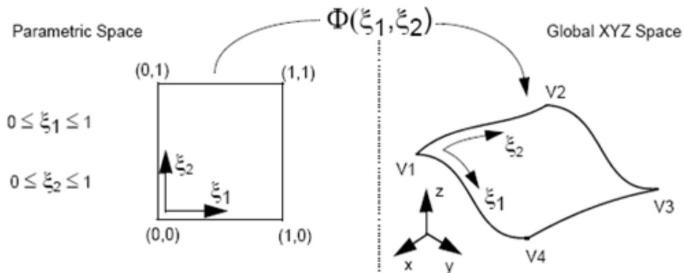
Figure 4-1 Mapping a surface from parametric space to global XYZ space
