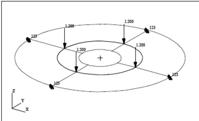
Figure 1-2 Patran Finite Element model of Annular Plate
