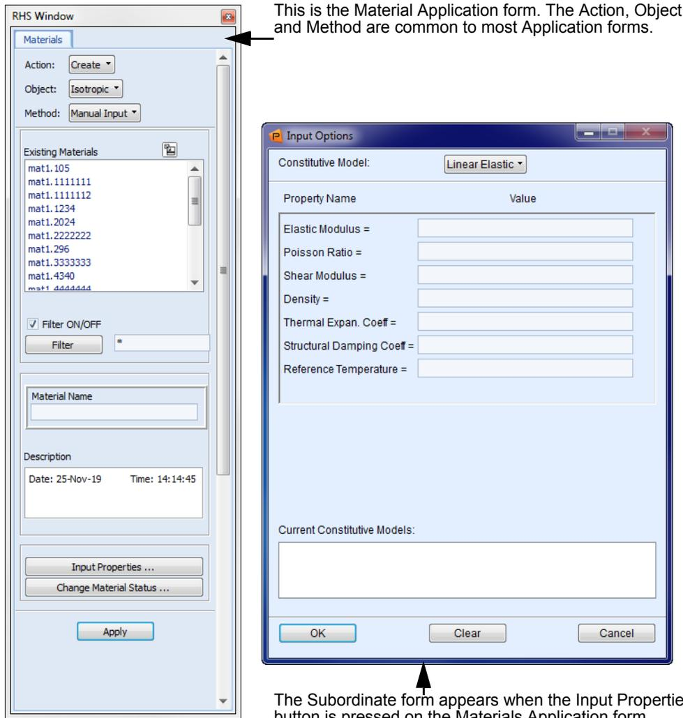
You can choose only one application radio button at a time. Once you pick a second application from the window, the second application form appears and the first form closes. While you can only have one application form open at a time, you can have other forms open from the menubar. The tabs located at the bottom of the forms allow you to toggle between the forms that you have open. You can close an application by clicking its radio button.
