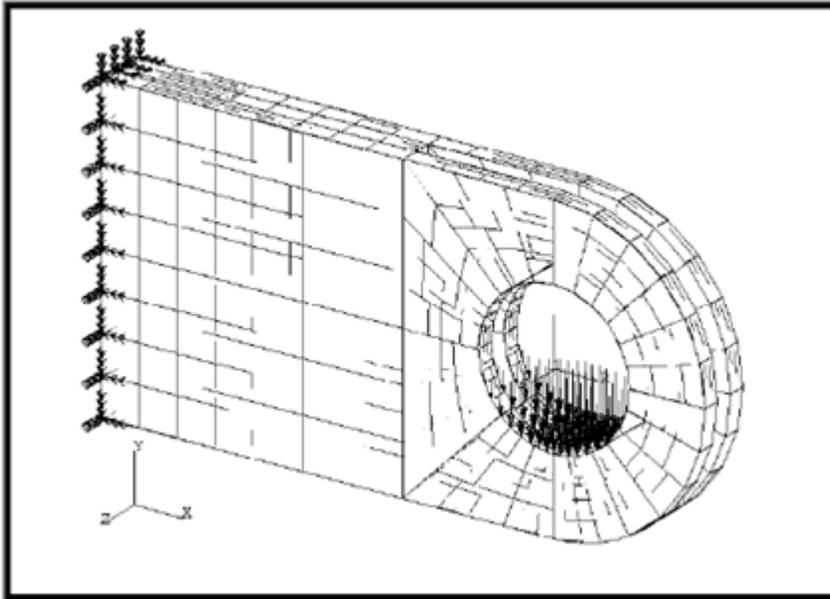
Figure 7-1 Model with point load and displacement boundary conditions
