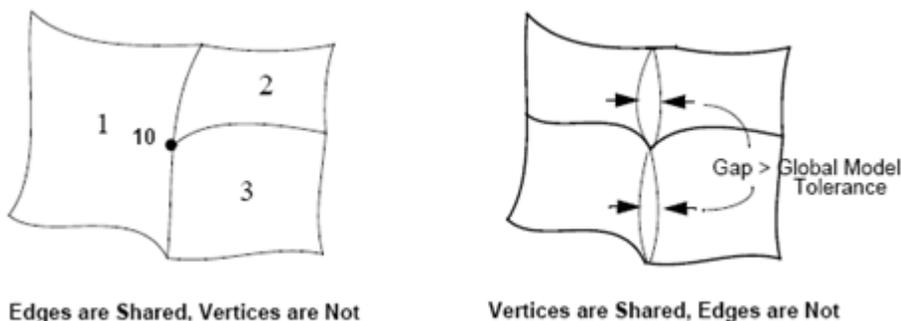
Figure 4-5 Noncongruent geometry with missing vertices
